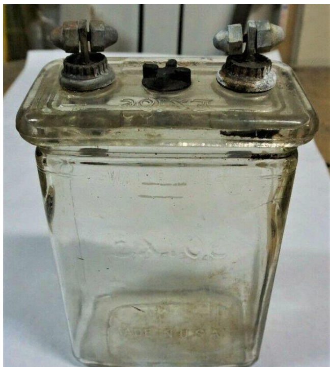
16.0.11 is reported to have been a radio battery. It is embossed EXIDE, with dimensions of 3" x 5" x 10" tall.
