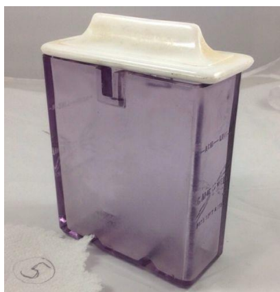
Gamewell glass battery jar with grooves in bottom.
